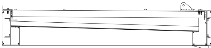
Gutter Forward With Scuppers
