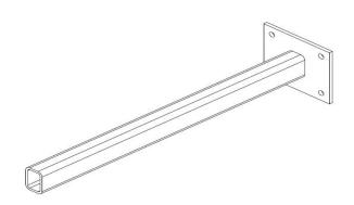
These are used for the Colorado and the Seattle systems. With a max projection of 4'-0". With the Seattle system the minimum face height must be 12". Max spacing is 5'-0".
